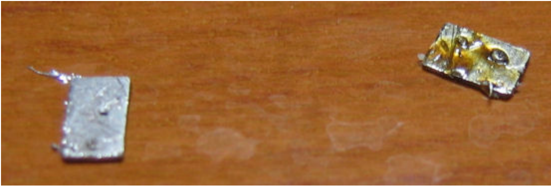
The metal plates soldered to the input pads on the protection board.
